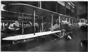
THE NEW CURTISS EAGLE CABIN PLANE IN COURSE OF ASSEMBLY, FLYING WITH TWO OF THE NEW CURTISS TWELVE 400-HP. ENGINES
